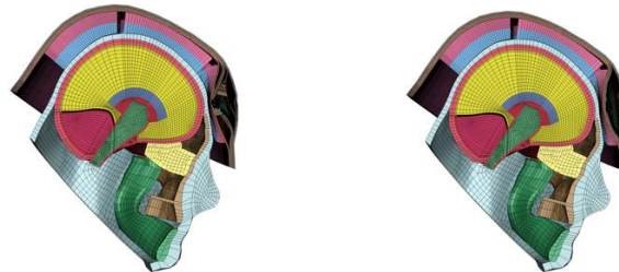
Figure 2: Deformation of the head protected with – Left: Kevlar helmet – Right: Dyneema helmet
