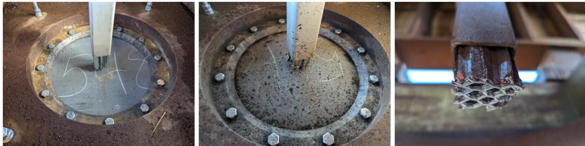
Figure 4: Crush block before and after testing
