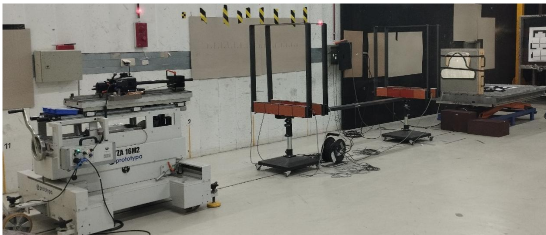
Figure 1 – Experimental setup used to evaluate the influence of under-vest fabric type on back-face deflection in a soft ballistic vest system.
