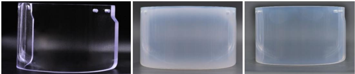
Figure 3: Visor before ageing - left, directly after the ageing (70 °C, 98 % RH for 2000 h) - centre, over a month after the ageing cycle - right
