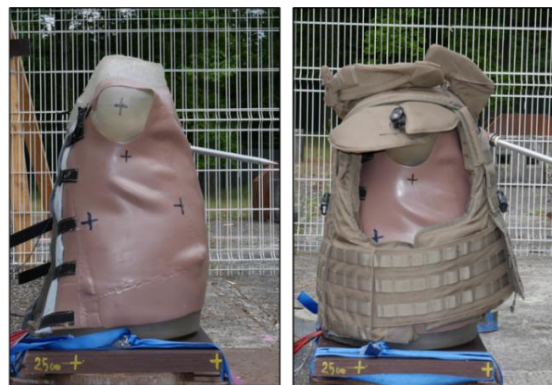
Figure 1: SurHUByx thoracic surrogate in two configurations: (a) without thoracic protective equipment (TPE), and (b) equipped TPE.
