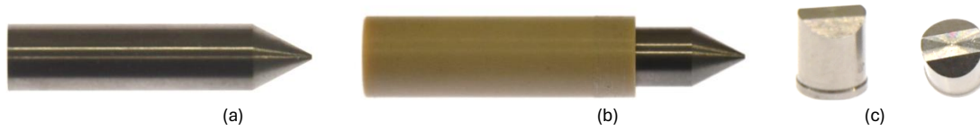
Figure 1. FOI:s test projectile (a) and when mounted in a plastic sabot of Duratron (b). The projectile length was 25 mm, the diameter 5.6 mm and the pointed 55° tip. The fragment simulating projectile FSP of mass 1.1 g (c).
