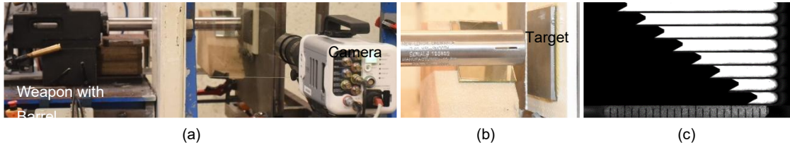
Figure 4: Test setup with the weapon with barrel and high-speed camera for the velocity measurement (a). The barrel with a slit (b) and examples of a pictures from the film for velocity measurement (c).
