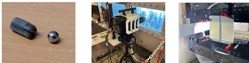
Figure 1: Rigid steel sphere used as projectile in the ballistic tests, followed by the high-speed camera used for recording and how the plate was clamped during the tests. [1].
