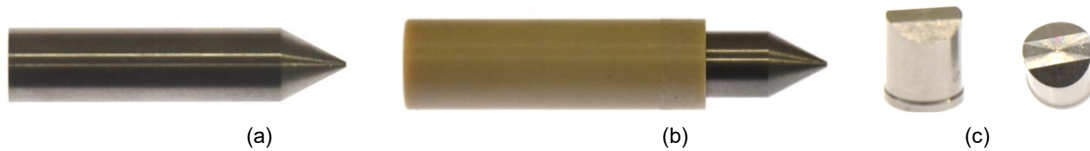
Figure 3. FOI:s test projectile (a) and when mounted in a plastic sabot of Duratron (b). The projectile length was 25 mm, the diameter 5.6 mm and the pointed 55° tip. The fragment simulating projectile FSP of mass 1.1 g (c).
