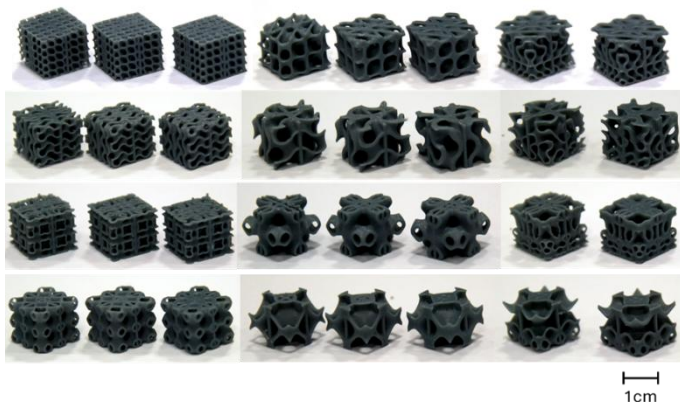
Fig. 1: Unit cells of miniaturised modified TPMS structures.
